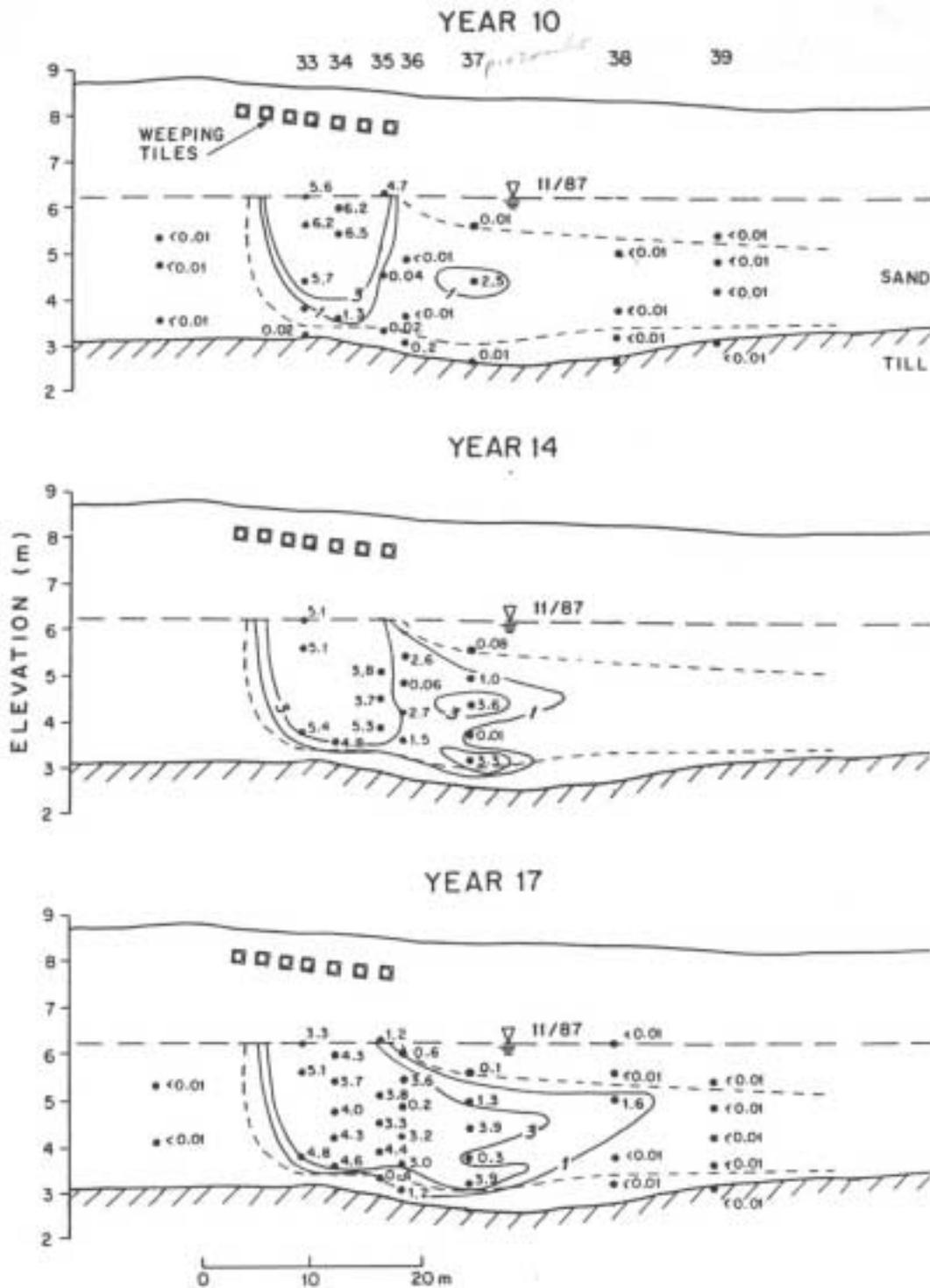
Figure 1. Phosphate distribution (mg/L) along the plume centerline during years 10 (1987) to 17 (1994) of system operation (dashed line denotes plume core based on Na<sup>+</sup> levels of >40 mg/L). (Robertson, 1995).
